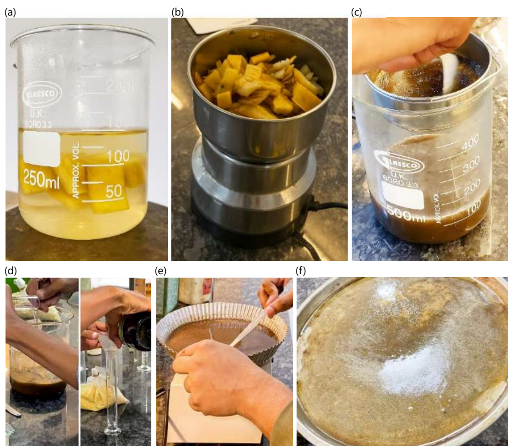
Fig. 3(a-f): Stepwise preparation of biodegradable plastic film from banana peels, (a) Chopped banana peels were put in a blender, (b) Boiled adding small amount of water, (c) Mixture strained using a strainer along with addition of gelatin, vinegar and glycerin, (d) Mixture heated at a medium flame, (e) Mixture poured on a glass petri plate and dried and (f) Material solidifies into biodegradable plastic films
